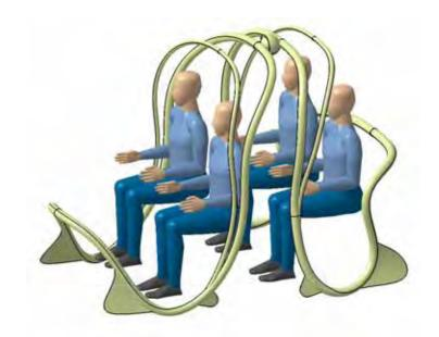
Dampening material placed between frame Side & front Ingress/Egress Twisting & Rocking frame – Dynamic Cabin
