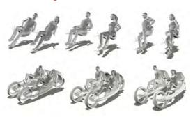
joints of the vehicle. Several movement studies were created to study the range of motion for controlling the car. This shows excerpts from one of the animation sequence that shows how the vehicle is constructed around the movement of the drivers.
