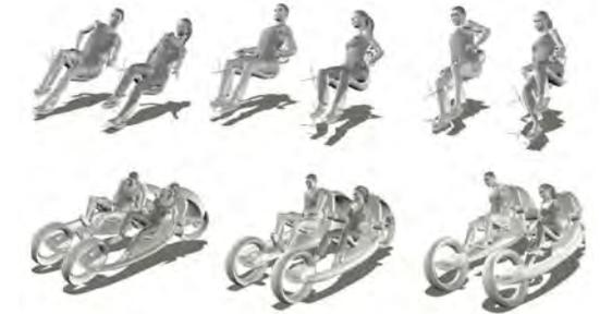
joints of the vehicle. Several movement studies were created to study the range of motion for controlling the car. This shows excerpts from one of the animation sequence that shows how the vehicle is constructed around the movement of the drivers.
